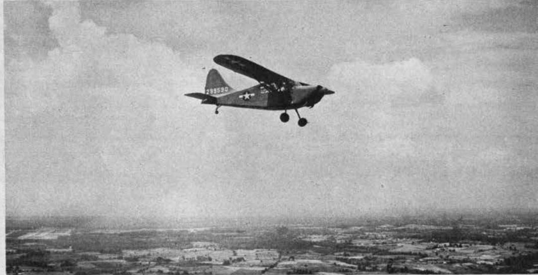
L-5B's thicker body (lower picture) may be contrasted with the tapering fuselage of L-5 (top). Though the change is important operationally, the two planes still look much alike.
